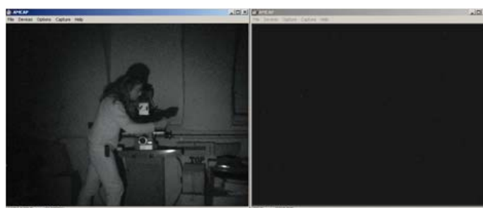
Figure 5. The IR-floodlight from Conrad makes everything clearer still. People are easily recognisable in complete darkness.
